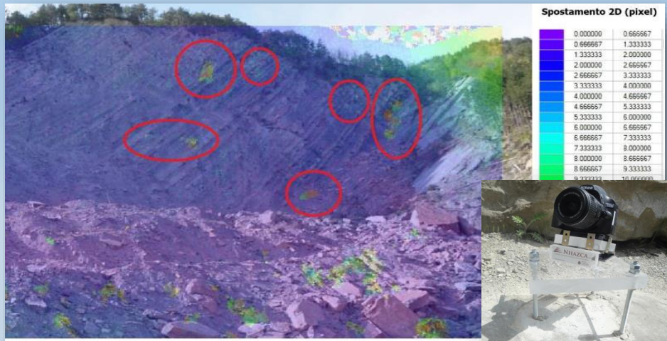
Digital Image Correlation (DIC) – Identificazione crolli
